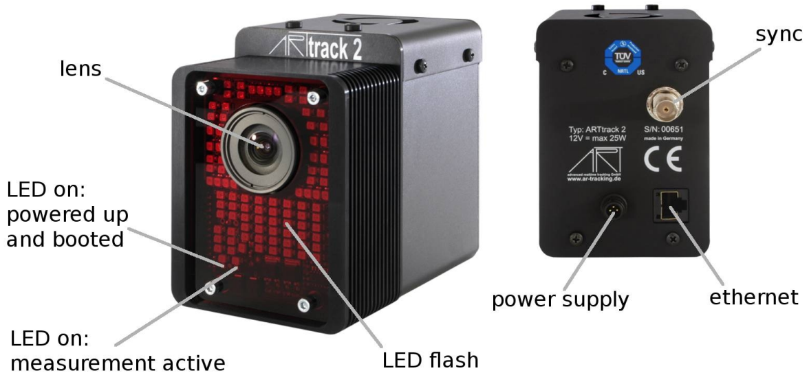
Figure 4.11: Camera ARTTRACK2 - Description of LEDs and interface connectors
