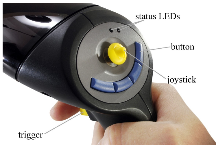
Figure 5.32: Flystick2 control elements
