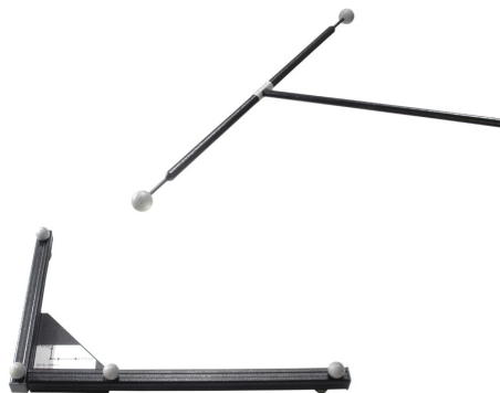
Figure 5.4: A room calibration set consisting of angle and wand
