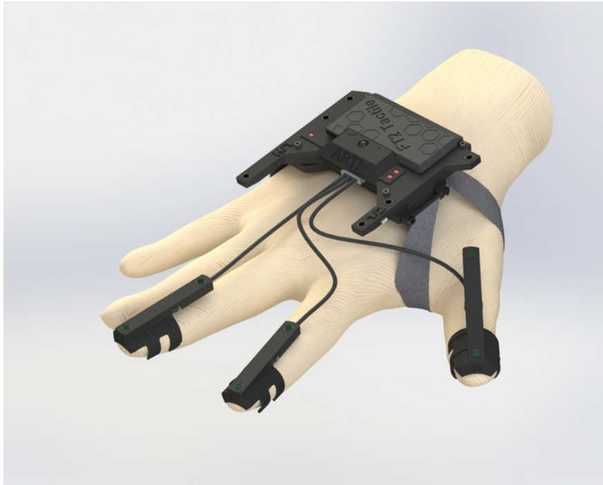
Figure 5.35: FINGERTRACKING2 and FINGERTRACKING2 Tactile device (shown with three active finger markers)
