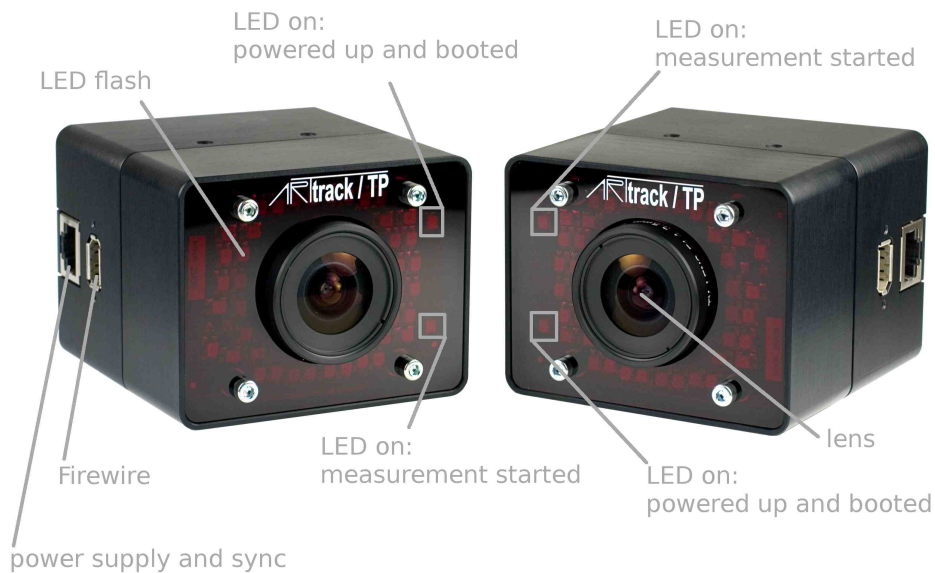
Figure 4.13: Camera TRACKPACK - Description of LEDs and interface connectors
