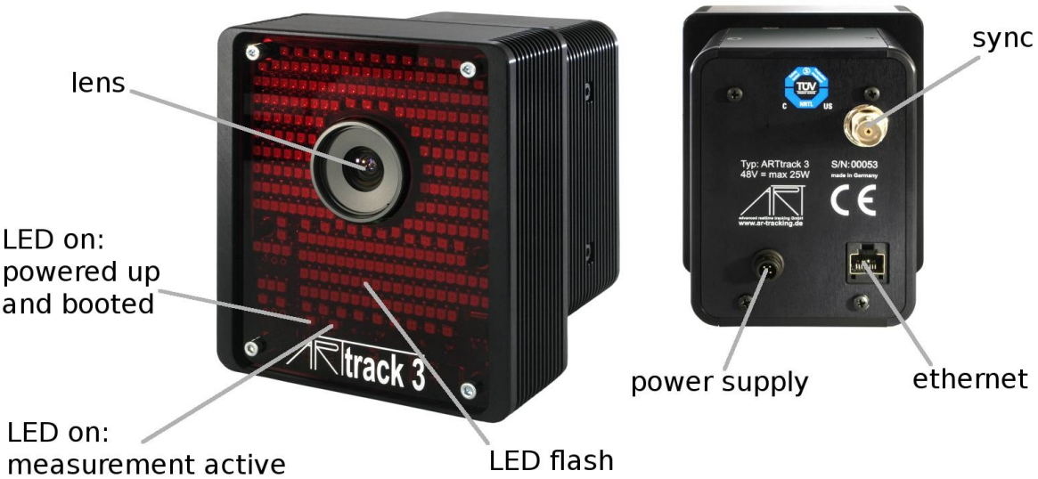
Figure 4.12: Camera ARTTRACK3 - Description of LEDs and interface connectors
