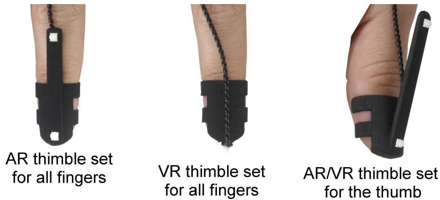
Figure 5.52: Comparison of the finger thimble sets (VR, AR) for Fingertracking (discontinued)
