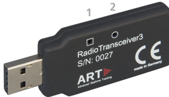
Figure 4.10: USB Radio Transceiver3 - Description of LEDs
