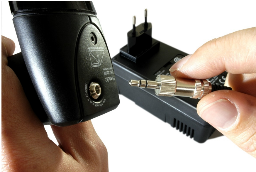
Figure 5.34: Charging the battery of the Flystick2
