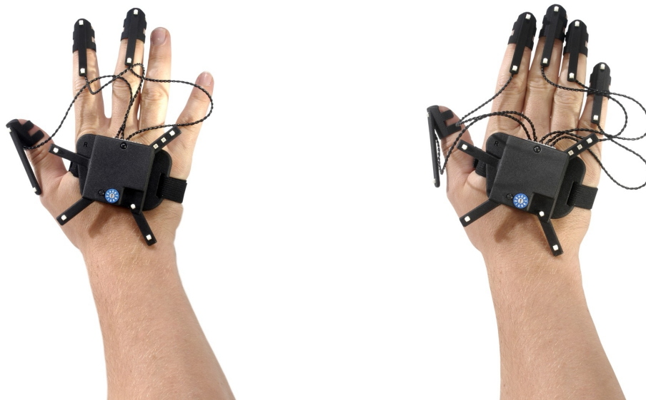
(a) Fingertracking device with three active finger markers
