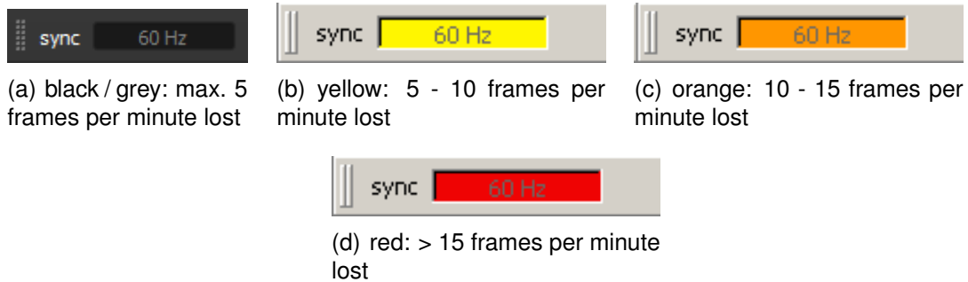
Figure 6.4: DTRACK3 3 Sync Status (toolbar element) - Visualization of the decrease in effective synchronization frequency
