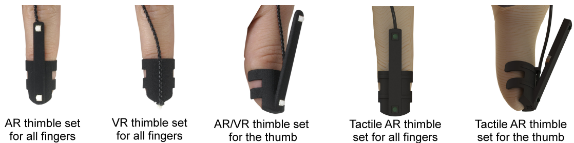
Figure 6.19: Comparison of the finger thimble sets (VR, AR) for Fingertracking and AR for FINGERTRACKING2 Tactile
